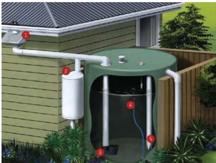
Screened rainhead, first flush diverter, calmed inlet, floating out-take and tank vacuum device. Reproduced with permission of David Oliver, Marley New Zealand.
